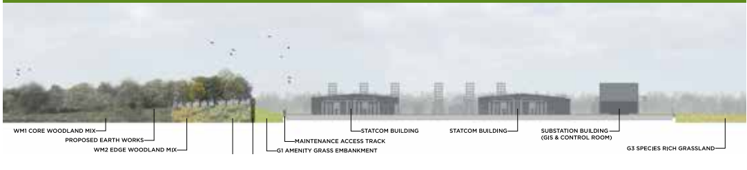
Cross section of East Anglia ONE substation and perimeter visual screening plan
